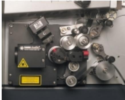
Unique in theatrical sound, the patented ERNEMANN® Laser Audio® optical soundhead offers full dynamic range with exceptionally clear, clean and bright sound quality. This is achieved by a highly concentrated red laser light which allows an effective slit height of only 6 micron on the film with precise edge-to-edge uniform illumination. Since the laser is controlled by APC (Automatic Power Control), the light intensity is kept
