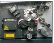
Unique in theatrical sound, the patented ERNEMANN® Laser Audio® optical soundhead offers full dynamic range with exceptionally clear, clean and bright sound quality. This is achieved by a highly concentrated red laser light which allows an effective slit height of only 6 micron on the film with precise edge-to-edge uniform illumination. Since the laser is controlled by APC (Automatic Power Control), the light intensity is kept absolutely constant. Thus, unlike
